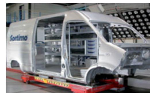
2004: sled test with Sortimo Globelyst in-vehicle equipment of the 3rd Generation with ADAC Bavaria
