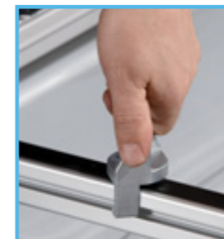
press the spring down and turn the hook ...
