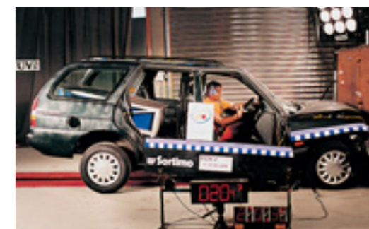
1986: sled test with Sortimo large drawer in a station wagon car
