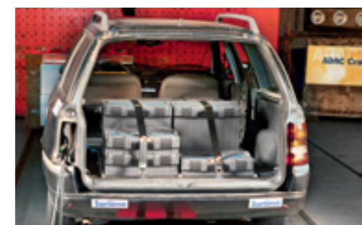
2009: ADAC crash test with Carmo floor plate and loaded and secured L-BOXXes with rear seat folded down at 50 km/h.
